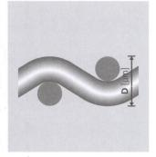
Mesh thickness D [µm] The mesh thickness **D** is measured according to ISO 5084.
