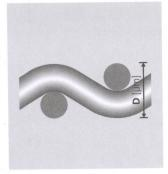
Mesh thickness D [μm] The mesh thickness D is measured according to DIN 53855-1. The tolerance is the defined range of the statistically ascertained mean values of mesh thickness.
