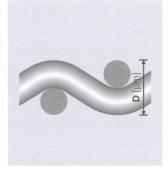
Mesh thickness D [ $\mu$ m] The mesh thickness D is measured according to DIN 53855-1. The tolerance is the defined range of the statistically ascertained mean values of mesh thickness.
