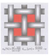
Percentage of open area  $\alpha_0$  [%] The percentage of open area  $\alpha_0$  is the sum of all mesh opening areas expressed as a percentage of the total screen area. It is calculated from the mean value of mesh openings and the actual diameter of the threads.
