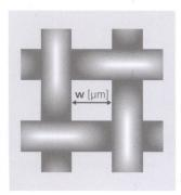
Mesh opening  $\mathbf{w}$  [ $\mu$ m] The mesh opening  $\mathbf{w}$  is the distance between two adjacent warp or weft threads.
